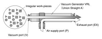
Select the proper type according to work-piece size and the amount.
